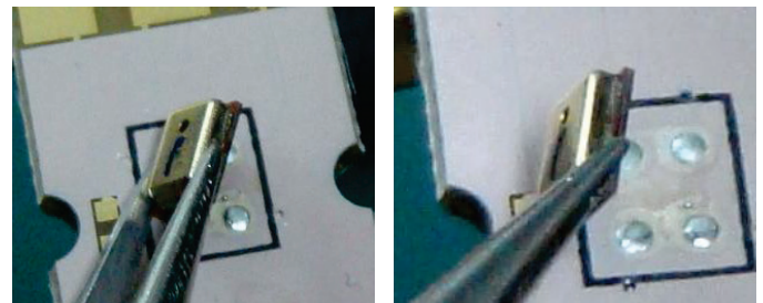
Figure 23. Improper (left) and proper (right) handling of microphones built using metal can construction
